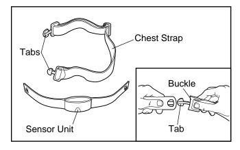
Next, wrap the heart rate monitor around your chest and attach the other end of the chest strap to the sensor unit. Adjust the length of the chest strap, if necessary. The heart rate moni-
